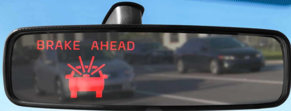
Electronic Brake Lamp Warning
